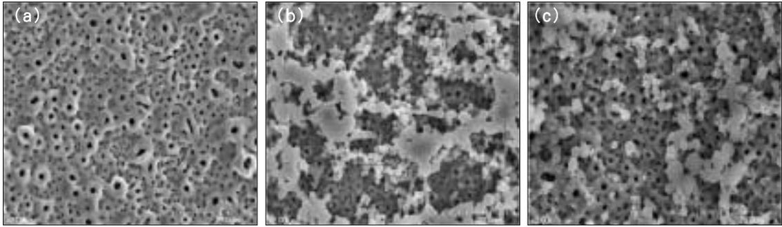
**Fig. 1.** SEM surface morphology of Ti disc surfaces (15 KV, 2.00 KX). (a) anodized surface, (b) PLGA coated surface, (c) PLGA and ZOL coated surface.
